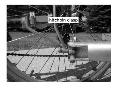
Place the towbar bushings on both sides of the ball of the rod end. Line up the holes so the hitchpin can fit down through the bushings and rod end. Take the hitchpin clip and swing it around behind the solid part of the towbar and stretch the clasp so it goes around the bottom end of the pin. You are now ready to use your trailer.
