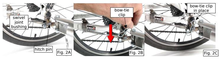
3. To remove the trailer from the hitch, pull the bottom of the bow-tie clip forward with your finger until it clears the hitch pin and push upwards from the bottom on the clip until the clip is out of the hole (Fig. 3).
